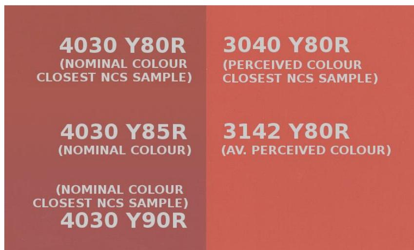
Figure 28: The nominal colour (left) and the average perceived colour (right) of façade F (Table 5).
