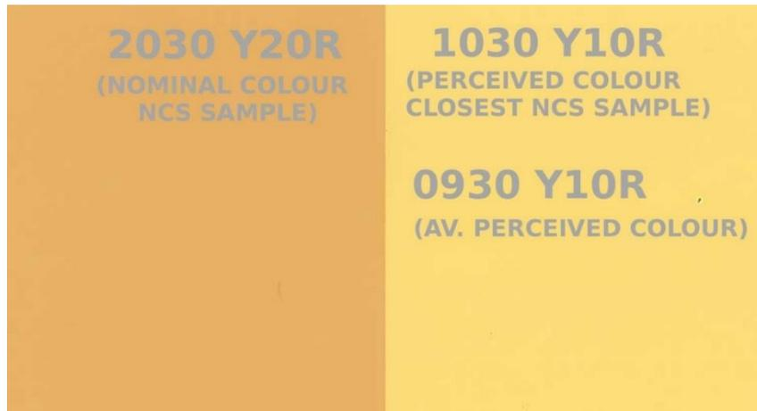
Figure 21: The nominal colour (left) and the average perceived colour (right) of façade B (Table 3).
