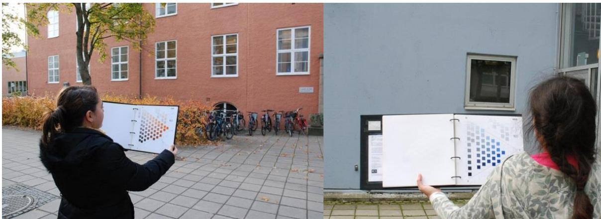
Figure 15: Illustration of the method for assessing perceived façade colour with the NCS Atlas. In the Warsaw study the distance between observer and façade was approximately thirty metres.
