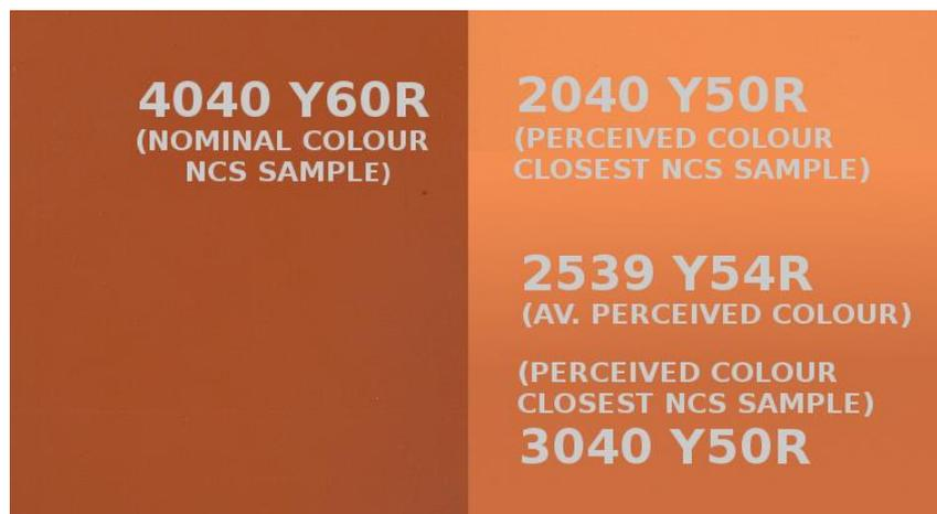
Figure 27: The nominal colour (left) and the average perceived colour (right) of façade D (Table 5).
