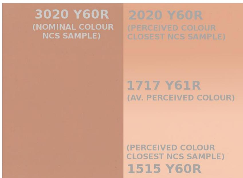
Figure 22: The nominal colour (left) and the average perceived colour (right) of façade G (Table 3).
