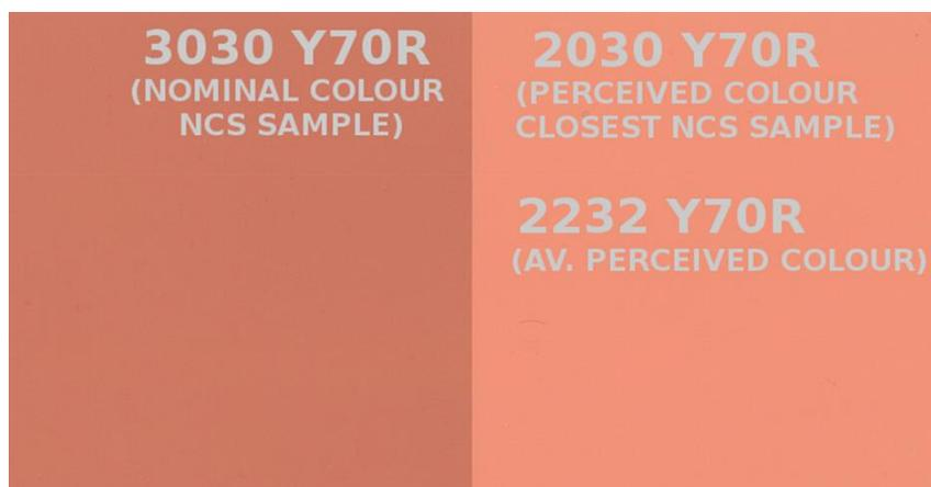
Figure 23: The nominal colour (left) and the average perceived colour (right) of façade H (Table 3).
