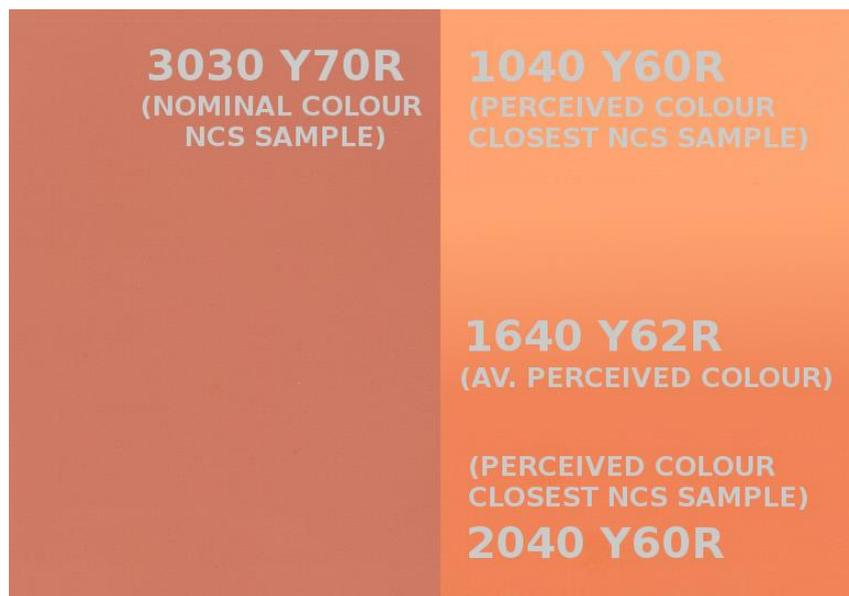
Figure 24: The nominal colour (left) and the average perceived colour (right) of façade I (Table 3).
